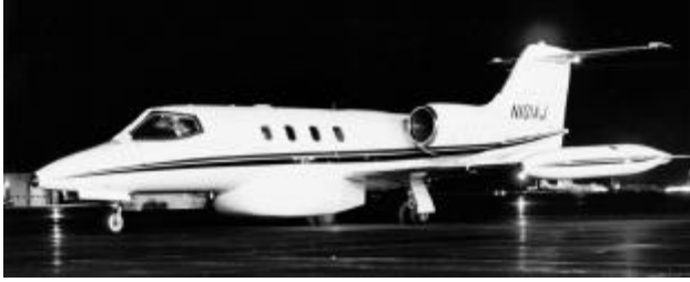
Figure 2: Learjet 36 Modified to Carry STAR-3i System
